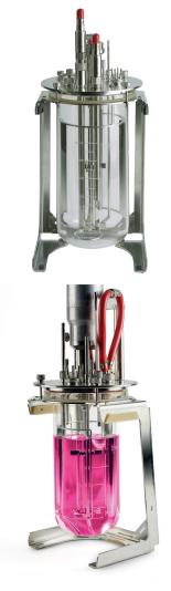
The F0-BABY bioreactor offers unmatched configurability, scalability, and robust software controls, all at an incredible price. Featuring versatile gas module options, interchangeable vessels up to 10L, and the ability to expand functionalities with external modules, this system empowers your bioprocessing endeavors. With software capabilities including recipes, profiles, dissolved oxygen cascade, and more, the F0-BABY is your gateway to enhanced productivity and flexibility.
